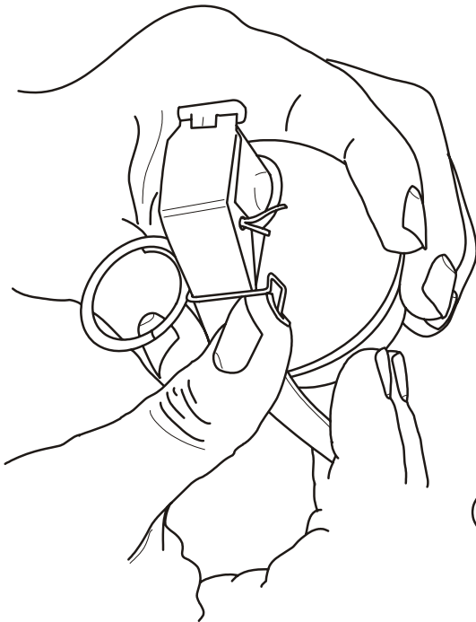
Figure 2-4. Assembly of safety clip to grenade M62.
